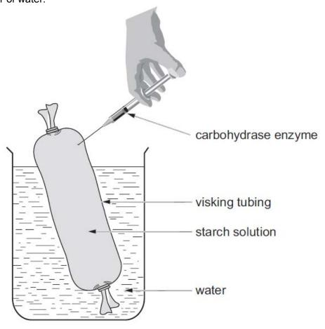
For the next 15 minutes the water in the beaker was sampled, at 5 minute intervals, for the presence of both starch and glucose. After 15 minutes a carbohydrase enzyme was injected into the visking tubing and further samples of water were tested.
